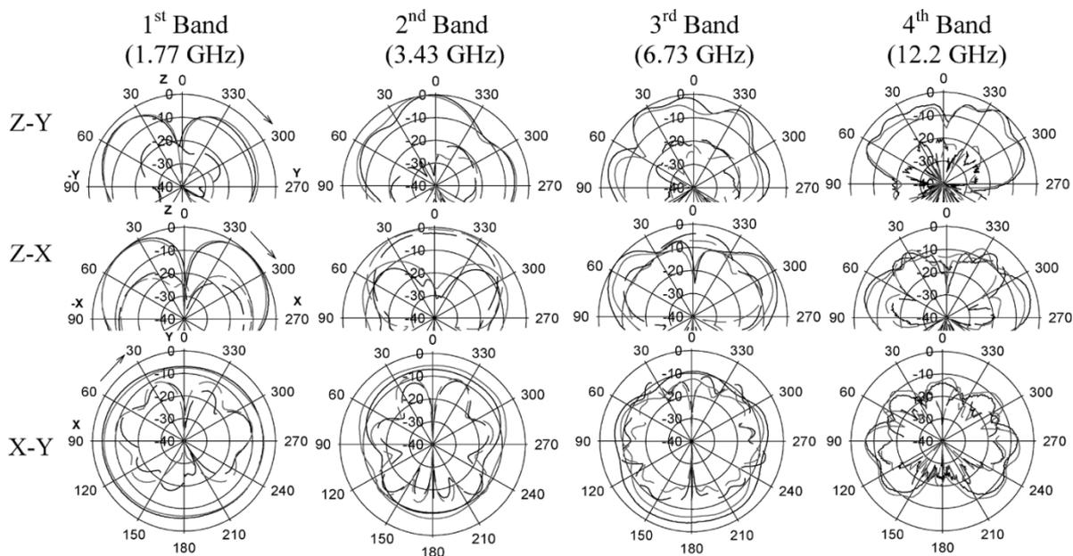
Fig. 5. Measured (black lines) and simulated (red lines) radiation plots of the vertically mounted folded shorted Sierpinski gasket antenna shown in Fig. 2 (— $E_{\theta}$ , - - $E_{\phi}$ ).
