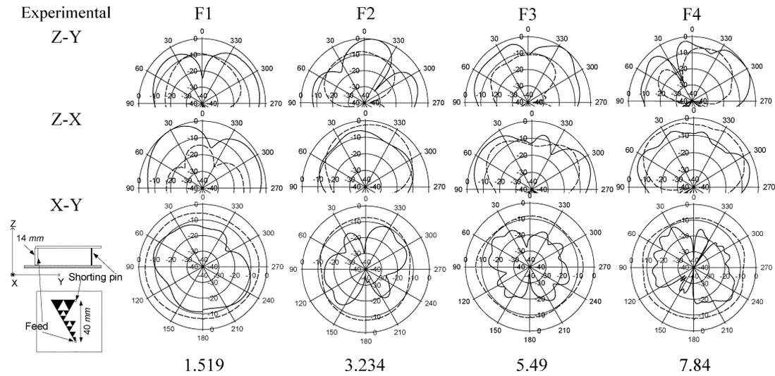
Fig. 8. Measured radiation pattern of the planar shorted Sierpinski gasket antenna shown in Fig. 6(a) (— $E_{\theta}$ , - -  $E_{\phi}$ ).
