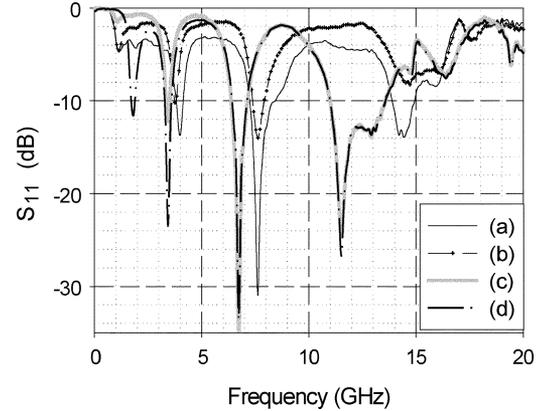
Fig. 3. Measured  $S_{11}$  comparison (a) vertically fed Sierpinski gasket shown in Fig. 1(a), (b) vertically fed halved Sierpinski gasket, (c) folded “inverted L” Sierpinski gasket shown in Fig. 2 with  $h_m = 5$  mm and shorting pin, (d) shorted folded “inverted L” Sierpinski gasket shown in Fig. 2 with  $h_m = 5$  mm.
