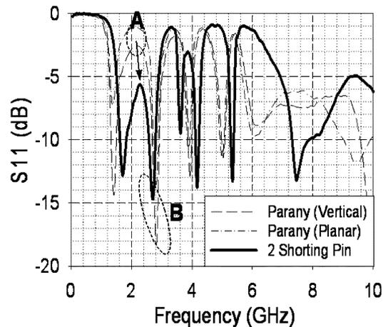
Fig. 11. Improved performance using two shorting pins.
