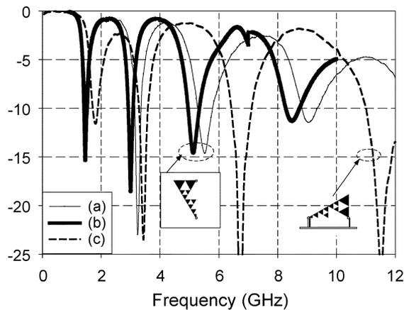
Fig. 7.  $S_{11}$  characteristics of the planar shorted Sierpinski gasket antenna: (a) measured, (b) simulated, and (c) vertical type configuration.
