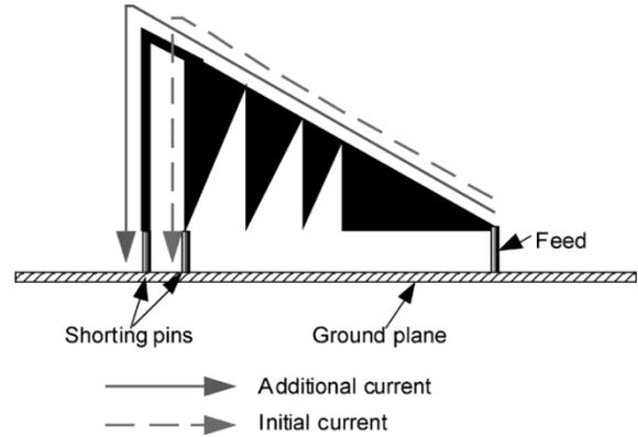
Fig. 10. Parany monopole antenna with dual shorting pins.
