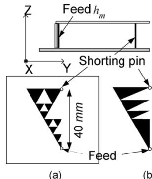
Fig. 6. (a) Configuration of the planar shorted Sierpinski gasket antenna and (b) configuration of the planar shorted Parany antenna.
