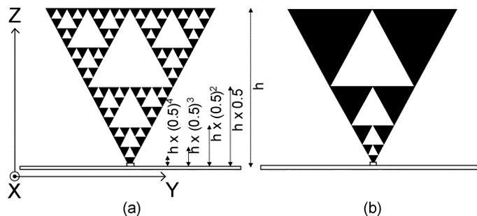
Fig. 1. (a) Fractal Sierpinski gasket monopole and (b) the Parany monopole antenna.
