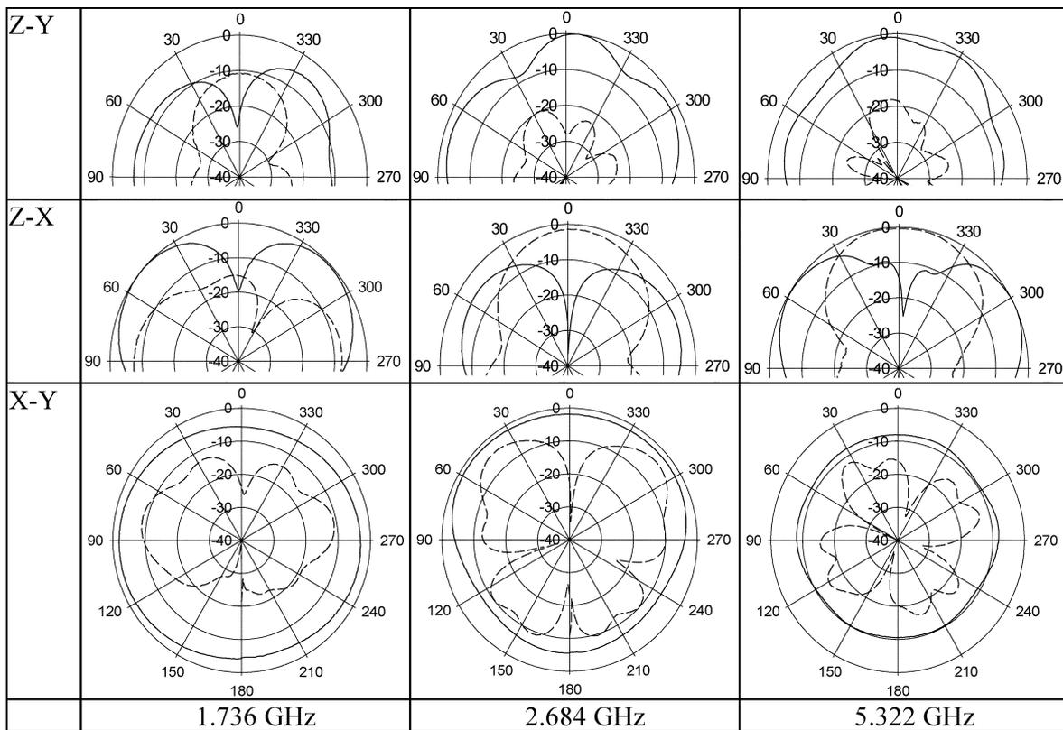
Fig. 12. Measured radiation pattern for the antenna shown in Fig. 10.
