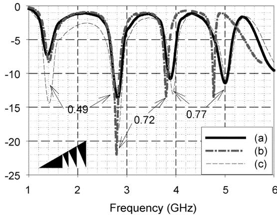
Fig. 9. Measured and simulated  $S_{11}$  characteristics of shorted Parany antenna shown in Fig. 6(b) (a) measured planar Parany, (b) simulated planar Parany, and (c) measured vertical Parany.
