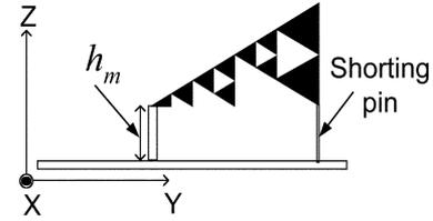
Fig. 2. Folded shorted “inverted L” Sierpinski gasket.
