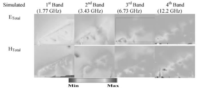
Fig. 4. Simulated field distribution of the four operating bands.
