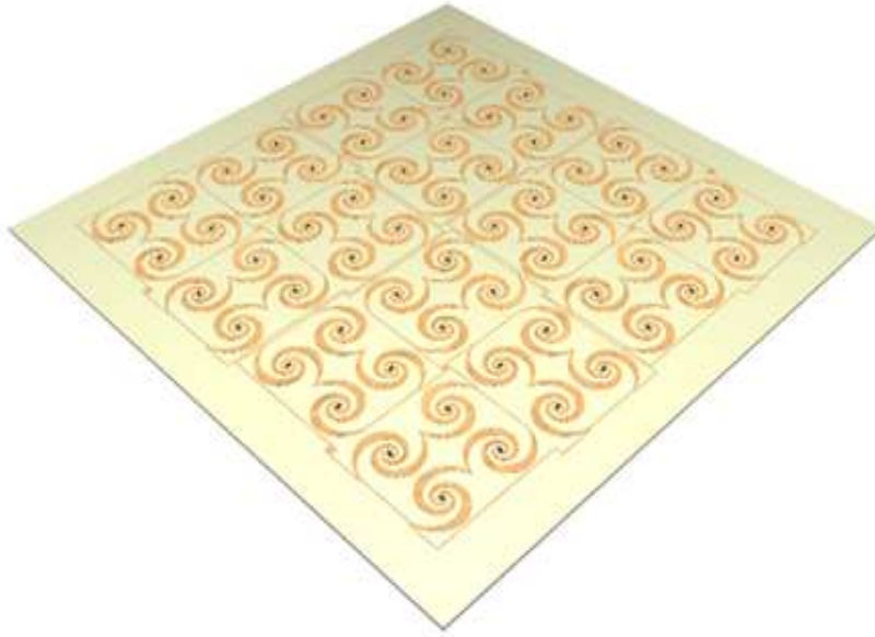
Figure 4.2: Layout of the 8 \times 8 array with 64 diodes (black devices), 4 \times 4 sub-arrays are not wired here, dimensions 185 \times 185 \text{ mm}^2
