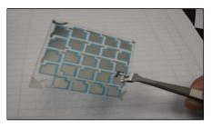
Figure 2: An organic semiconductor-based small molecule solar cell series array developed in the Columbia Laboratory for Unconventional Electronics (CLUE).
