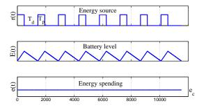
Figure 4: Application of the *Economic Production Quantity* (*EPQ*) model to the EnHANTs domain with a periodic on/off energy source: (i) the energy charge rate r(t), (ii) the energy level E(t), and (iii) the energy consumption rate e(t).
