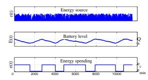
Figure 5: Application of the *order-point*, *order quantity* (s, Q) inventory model to the EnHANTs domain: (i) energy charge rate r(t), (ii) the energy level E(t), and (iii) the energy consumption rate e(t).
