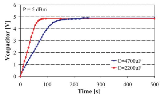
Figure 5. Charge of  $4700\ \mu\text{F}$  and  $2200\ \mu\text{F}$  energy buffer with  $5\text{ dBm}$  of input power at antenna.
