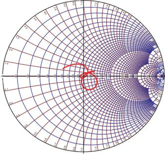
Figure 2. Input impedance varying the input power from  $-15\text{ dBm}$  to  $10\text{ dBm}$ .
