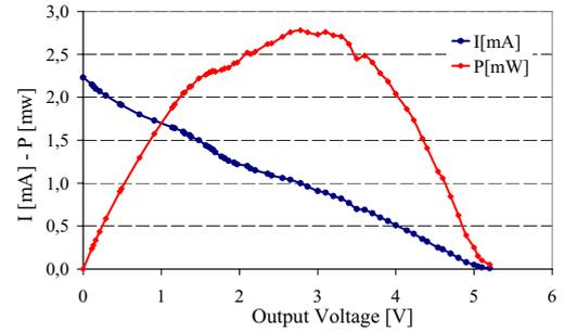
Figure 3. Characteristic of the harvester with  $5\text{ dBm}$  of input power
